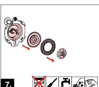
7. • Clean the shaft, gasket and exhaust opening.
