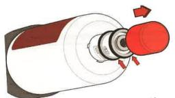
7. Remove protective cap from top of new cartridge and moisten o-rings with water and ensure the they are in place.
