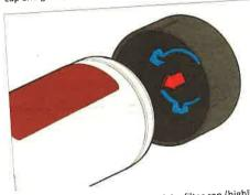
5. Align the shape on the inside of the filter cap (highlighted above) with the shape on the end of the new filter and push the two together until it clicks firmly in place.
