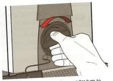
3. Grip Cartridge and rotate a quarter turn to the left and pull forward. CAUTION: A small amount will drain from the head and be directed to the front drip-tray as cartridge is removed.
