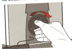
8. Insert new cartridge and turn until it locates. Install with a quarter turn to the right until cartridge comes to a complete stop (Inlet water will automatically turn on)
