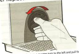
Grip Cartridge and rotate a quarter turn to the left and pull forward. CAUTION: A small amount will drain from the head and be directed to the front drip-tray as cartridge is removed.
