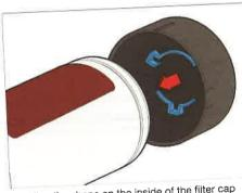
6. Align the shape on the inside of the filter cap (highlighted above) with the shape on the end of the new filter and push the two together until it clicks firmly into
